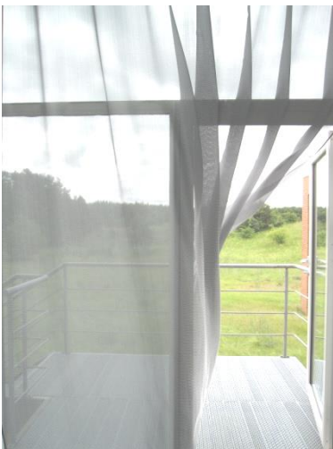
Figure 94 Picture used to illustrate three parameters influencing textiles effect on light: the importance of number of layers, distance between layers and density of the textile. Photograph: © Elisabeth Heimdal.
