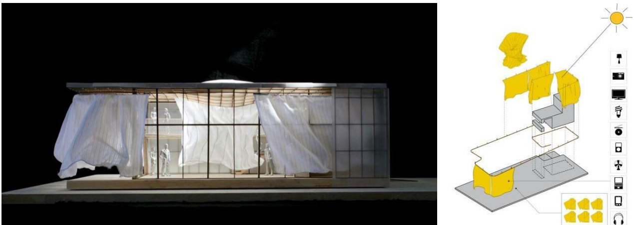
Figure 36 Soft House by Sheila Kennedy. Kennedy developed the project from the research department of her studio KVA MATx together with a team of architects, engineer, fabricators and manufacturers. Left: Physical model of the soft house. Both the central curtain and the curtains positioned along the windows are visible. Right: Illustration showing the curtains in yellow. These are imagined to be harvesting energy from the sun that is then distributed to the electrical appliances in the house and they can be positioned in different ways as shown in the lower right corner of the illustration. Source (for both images): (Kennedy, 2011b).
