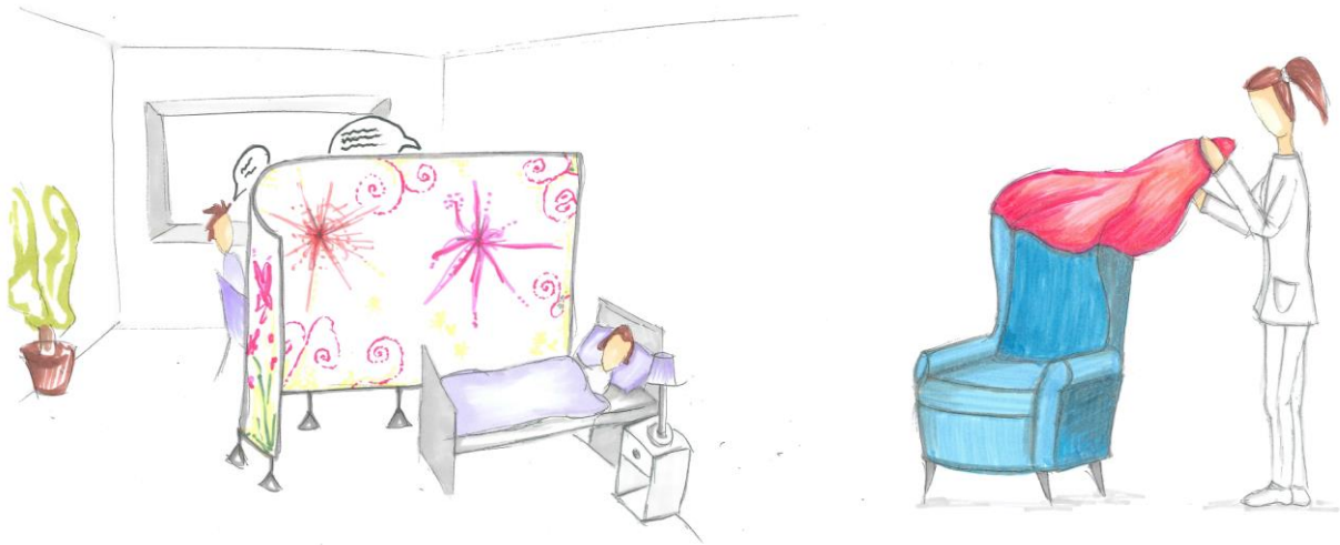
Figure 67 The two ideas chosen to be developed further in Design:Lab 2 by the patient ward group. Left: Movable partition wall with changing patterns and acoustic properties. The idea is that the pattern changes as a reaction to sound, while at the same time absorbing sound. Right: Removable upholstery cover for comfortable chair for relatives.
